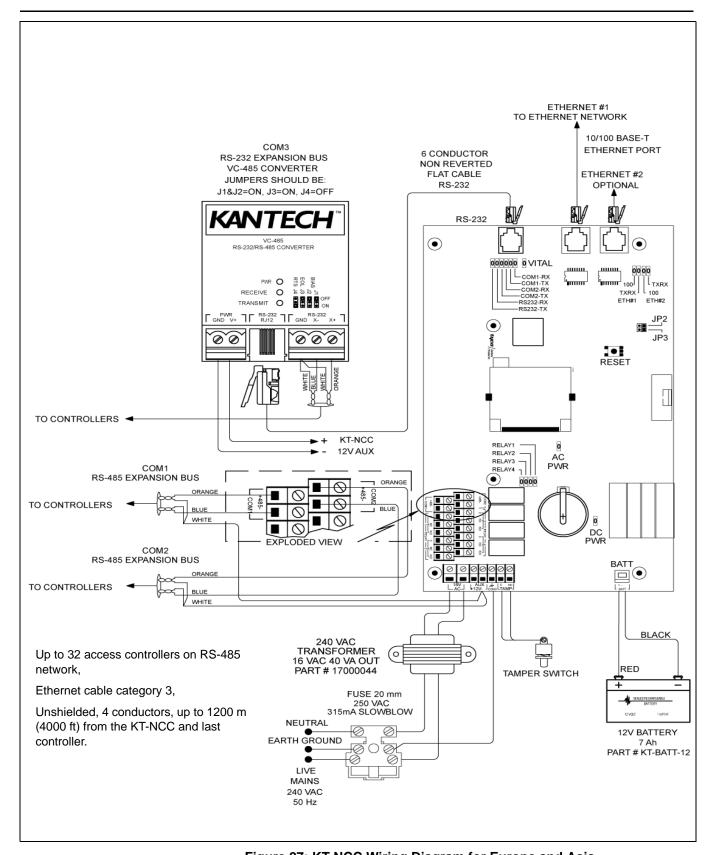
Figure 27: KT-NCC Wiring Diagram for Europe and Asia
