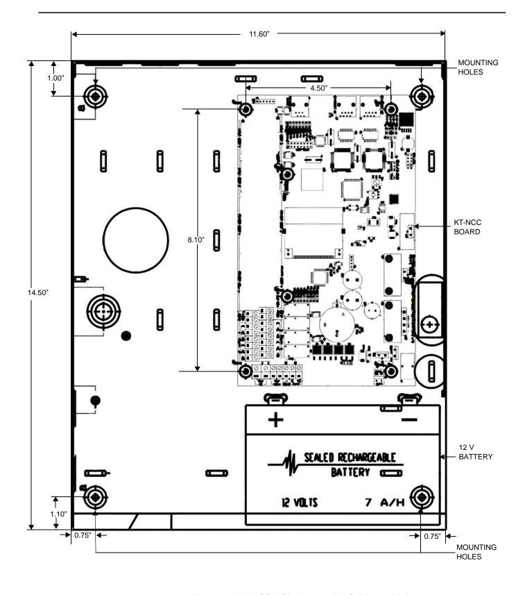
Figure 28. KT-NCC PCB Mounted in Cabinet with Battery
