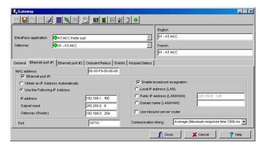
Figure 21. Gateway Window - Ethernet #1 Tab Static IP Address
