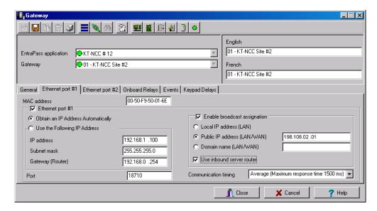
Figure 24. Gateway Window - Ethernet #1 Tab WAN
