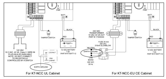
Figure 3. Tamper Switch and Earth Grounding
