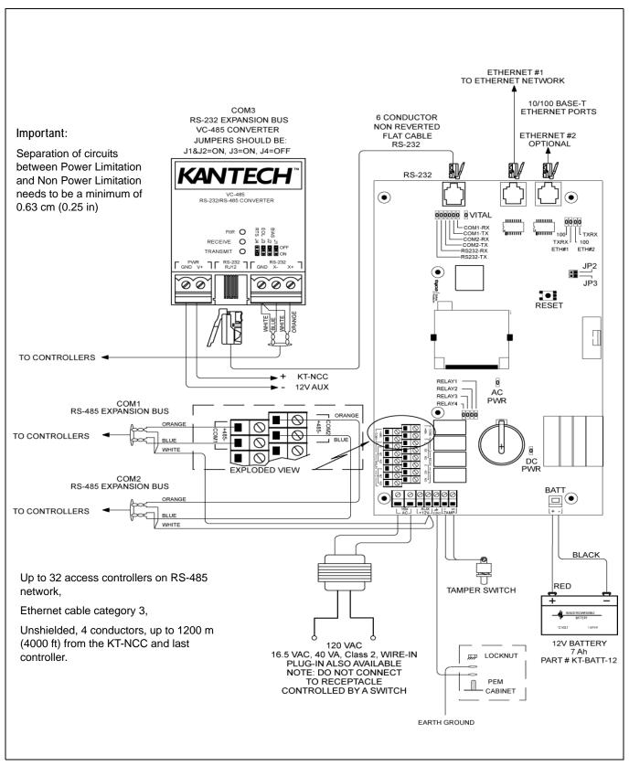
Figure 26. KT-NCC Wiring Diagram for North America
