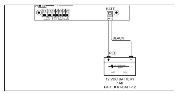
Figure 8. Connecting the Battery
