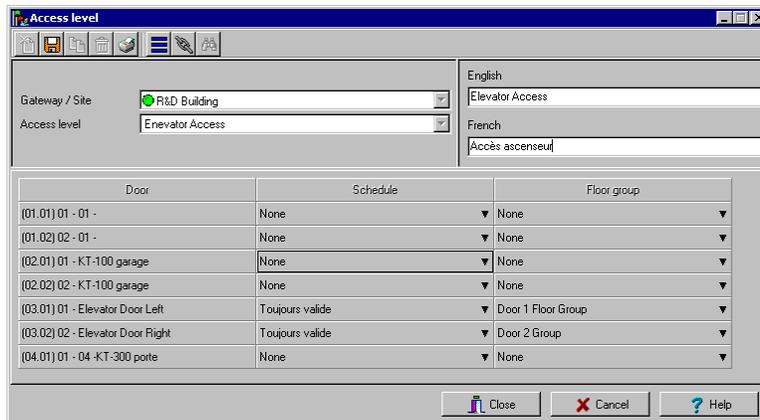
27. Near the end of the setup process, you may now enable access control on both Elevator door #1 and Elevator Door #2. To do so, simply assign one of the default schedules and a floor group to each elevator door.
