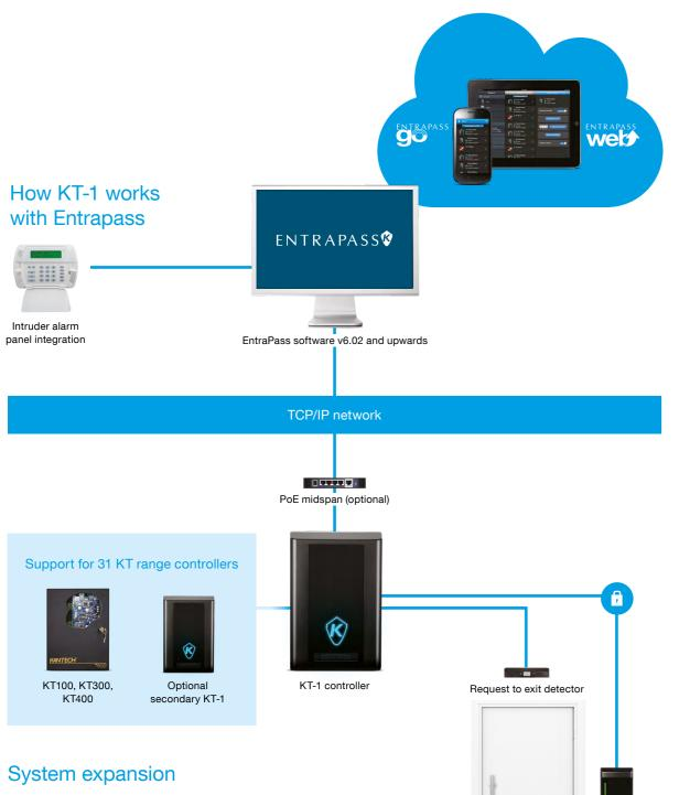
Not only can you connect hundreds of KT-1 controllers in one access control system, but a single KT-1 controller can also act as a 'head IP Controller' for more than 31 additional controllers under one IP connection in EntraPass.
